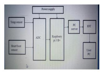
Fig 4: Block diagram of proposed system
