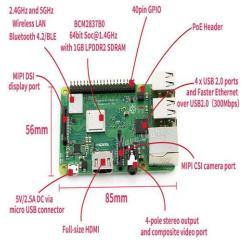
Fig 1: Raspberry pi 3 model B+
