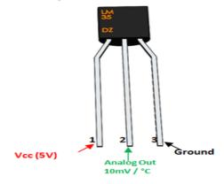
Fig 3: Temperature sensor
