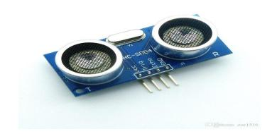
Fig 4.Ultrasonic Sensor
