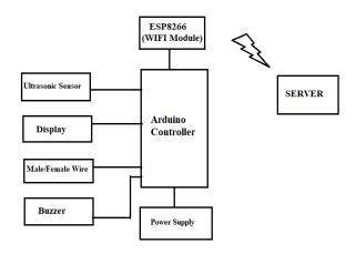
Fig 2. Block Diagram
