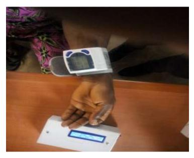
Fig 7 : HBR, BP and Temp Measurement with the Constructed Wireless Monitoring Device.
