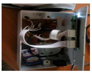
Fig 5 : The Wireless Monitoring Device Receiver
