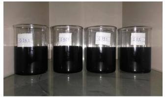
**Fig.4-** Nano lubricants of different mass concentration of CuO nano particles
