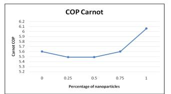
**Graph -1: Carnot COP Vs Percentage of nanoparticles** After experimentation, COP with pure POE oil is found to be 5.6 and with nanoparticles of 0.25% and 0.5%, COP is 5.489 and 5.5 respectively. So with the nanoparticles of 0.75% and 1% Carnot COP was increases 5.600 and 6.060 respectively. **3.5. Effect on Theoretical COP:**
