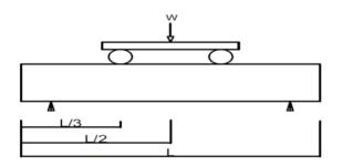
Beams were tested in UTM by Two-point loading method with an effective span of 800mm. Two Dial gauges were used to measure the deflection. The testing was carried out in 1000kN capacity UTM. Two-point load were applied and displacement of the beam specimen were noted.
