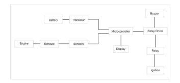
When the emission level is above 90% the microcontroller sends signal to the relay module which is connected to the ignition and shutdowns the power in the ignition and the power supply to the vehicle is cut off.
