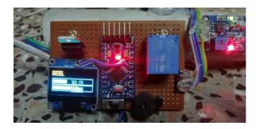
There is and switch that switches the module from petrol to diesel or diesel to petrol.
