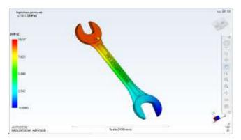
Fig 4.8 Injection pressure at gate location 2
