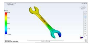
Fig 4.7 Injection pressure at gate location 1
