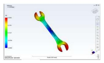
Fig4.1: Fill time of gate location 1
