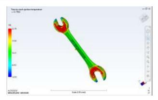
Fig.4.5 time to reach ejection temperature at gate 1
