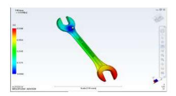
Fig.4.2:Fill time of gate location 2
