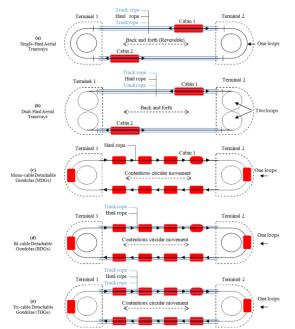
Fig -3: Detailed illustrations of RTS technologies IRJET
