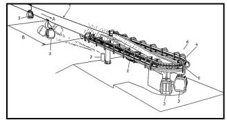
Fig -2: Turning point station
