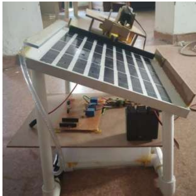
Figure 2.6: Whole System (side view)
