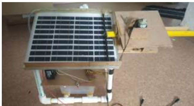
Figure.2.1: Working model of Automatic Solar Panel Cleaning System
