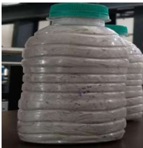
Figure 4: Waste Plastic compacted in bottles
