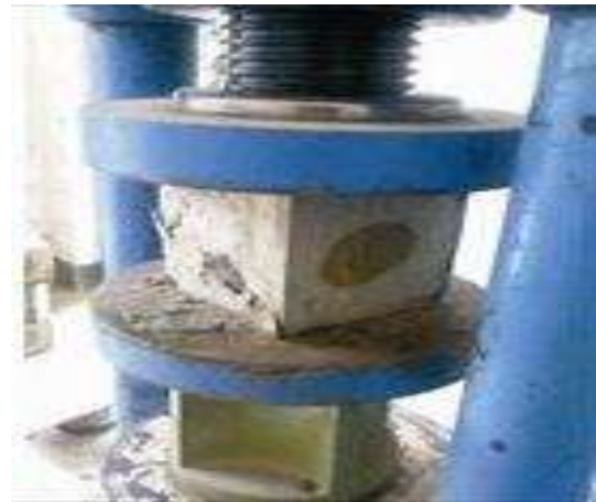
Figure 5: Compression test on Concrete Cube
