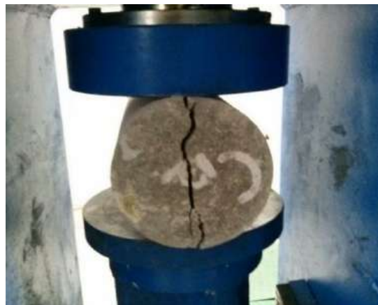
Figure 6: Split Tensile test on Concrete
