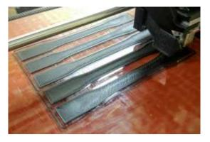
Fig -2: Specimens Manufacturing
