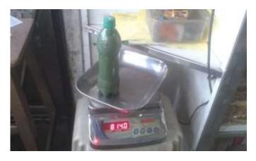
Fig 2: Weighing Balance to weight pet bottle before testing
