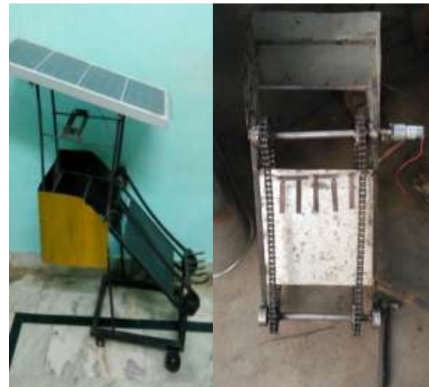
Fig. Construction of river cleaning machine
