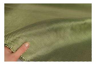
As an anisotropic material, it's transverse and shear modulus are an order of magnitude less than those in the longitudinal direction. The fibers can have difficulty achieving a chemical or mechanical bond with the resin.
