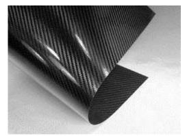
The most frequent additive is silica, but other additives such as rubber and carbon nanotubes can be used. CFRP are commonly used in the transportation industry, normally in cars, boats and trains, and in sporting goods industry for manufacture of bicycles, bicycle components, golfing equipment and fishing rods.
