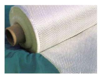
The fibers are drawn into very fine filaments with diameters ranging from 2 to 13 X 10<sup>-6</sup> m. The glass fiber strength and modulus can degrade with increasing temperature. Although the glass material creeps under a sustained load, it can be designed to perform satisfactorily. The fiber itself is regarded as an isotropic material and has a lower thermal expansion coefficient than that of steel.
