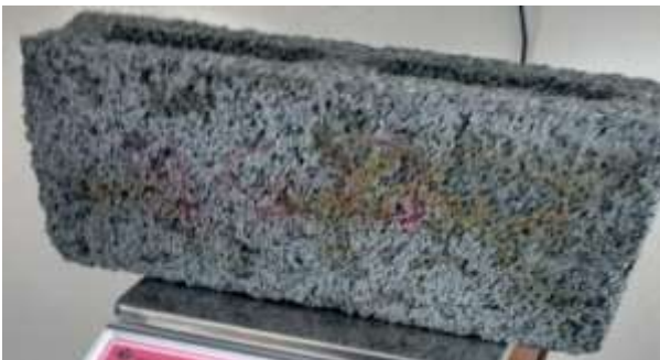
Fig 4.52 Acid attacked block
