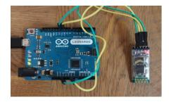
Fig -3: Bluetooth HC-05 and Arduino
