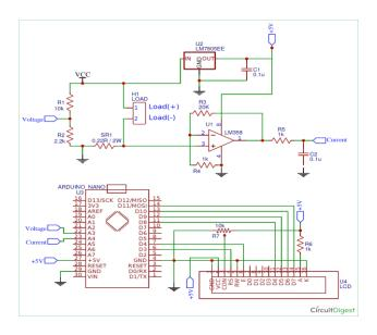
Fig -5: Schematic diagram
