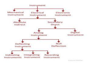
**Fig -1**: Classification of Instruments
