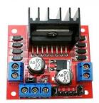
The L298N motor controller follows the H-bridge configuration, which is handy when controlling the direction of rotation of a DC motor. It is ideal for robotic applications and well suited for connection to a microcontroller and raspberry pi requiring just a couple of control lines per motor. The L298N has four inputs corresponding to the four switches. All
