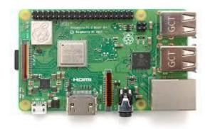
The Raspberry Pi is a cheap, credit-card sized computer that plugs into a computer monitor and can be used with a standard keyboard and mouse. It works as a desktop computer and can be use to learn programming, build different hardware projects, do home automation and even use in industrial application. It provides a set of GPIO pins that allow you to control electronic components and explore IoT.
