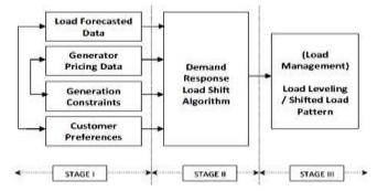
**Fig.2:** Basic working model of Automatic Demand Response
