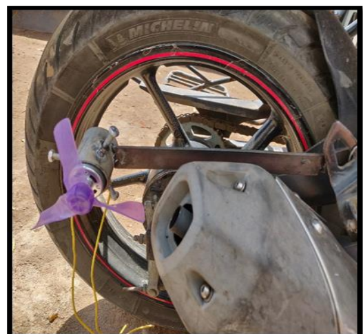
Fig -3: setup of generator rotor on Bike
