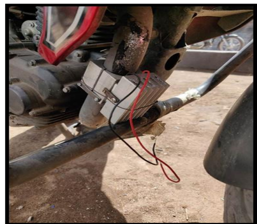
Fig -2: setup of thermoelectric generator on Bike
