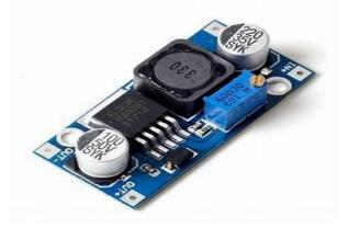
XL 6009 dc-dc booster is used to increase the output current from capacitor of 2.7V to 9-12 Volts which can run four motors of 3 volts.
