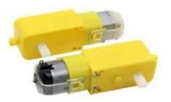
3 Volts single shaft geared motor is used as hub motor for prototype made. This motor as 150 rpm at no load condition. This motors operate at 3v-9v.
