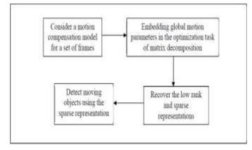
Fig -8: Concept of Low Rank & Sparse decomposition technique for moving camera [24].
