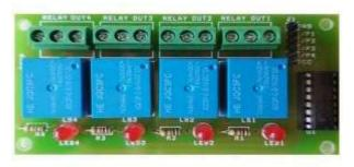
A relay is an electromagnetic device managed by a comparably small electric current that can turn on or off a much larger electric current. A relay has NO and NC states. When a relay is empowered it switches from NO to NC or from NC to NO whatever its previous state be.
