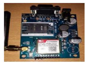
The GSM stands for GLOBAL SYSTEM for MOBILE COMMUNICATION.GSM module is a chip or circuit that is used to establish communication between a mobile device and a GSM system.
