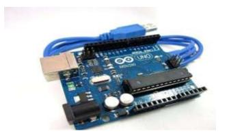
The Arduino Uno board is a microcontroller based on the ATmega328. It has 14 digital input/output pins in which 6 can be used as PWM outputs, a 16 MHz ceramic resonator, an ICSP header, a USB connection, 6 analog inputs, a power jack and a reset button.
