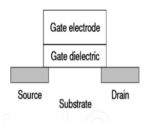
Fig.1 Schematic of high K dielectric based MOS [5].
