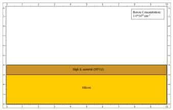
Fig.2 Deposition of high k-dielectric layer (HFO2).
