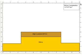
Fig.3 Etch out the extra material.
