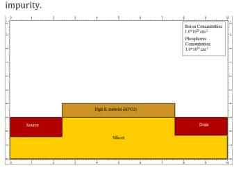
Step: 4 Drain and source is created using phosphorus
