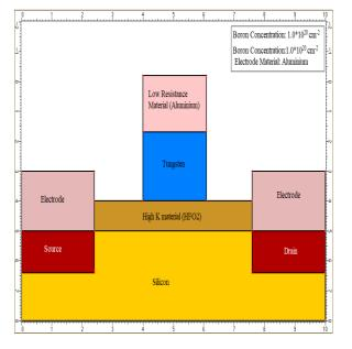
Fig.7 High k-dielectric based device.
