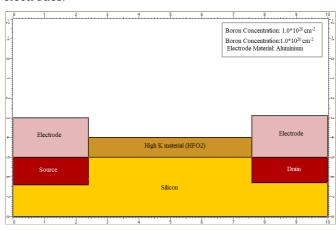
Fig.5 Electrodes are deposited
