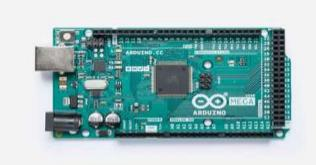
Fig -2: Arduino Mega
