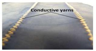
Fig -5: Conductive Yarn
