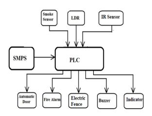
Fig-1: Smart Bank Security Using PLC
