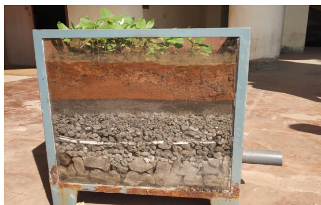
Fig .1(a) Vertical filter bed
