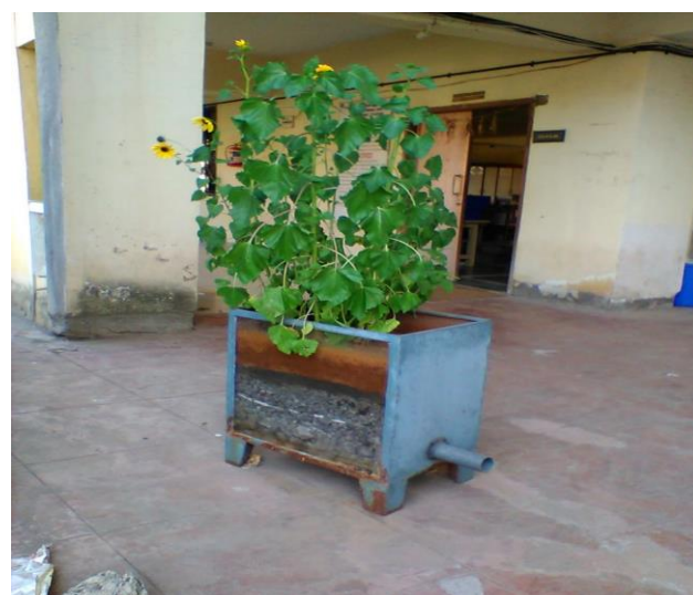
Fig .1(b) Vertical filter bed with sunflower plants
