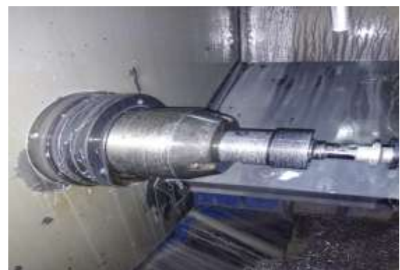
Fig 6. Fixture mount on CNC machine
