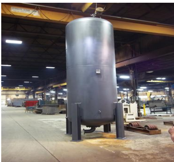
Fig1.8 Lug support for vertical[8]
