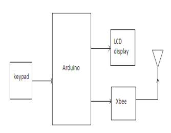
Fig: Block diagram of transmitter
