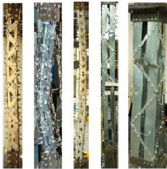
Fig-7: Various modes of failures observed.
