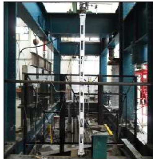
Fig-1: Test setup for the built-up cold-formed steel section battened column.
