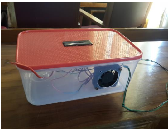
Fig-11: Final prototype of Smart Incubator with Real Time Temperature and Humidity Control
