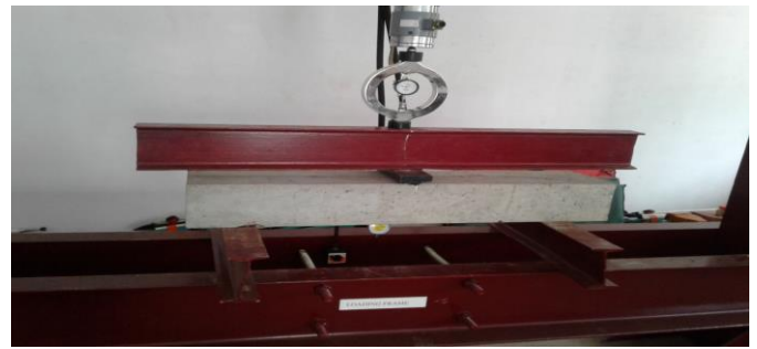
Fig -6: Experimental setup for testing of RC beam
