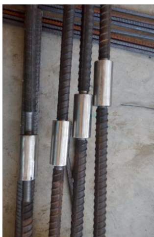
Fig -5: Steel with Bar Coupler
