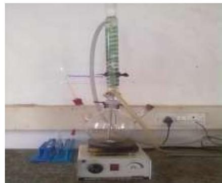
Fig -4: Experimental Trans-esterification setup
