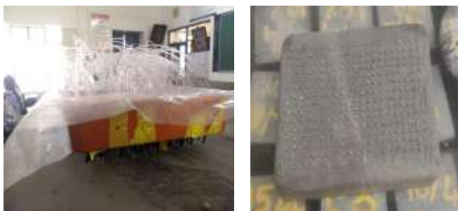
Fig -5.1: Sun light passing through the LITRACON BLOCK (Picture: during day time)
