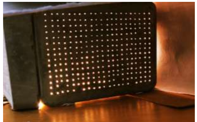
Fig-5.2: Light transmitting panel making using optical fibers
