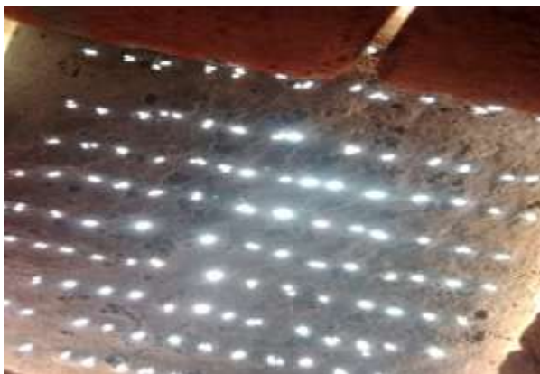
Fig -5.1: Sun light passing through the LITRACON BLOCK (Picture: during day time)
