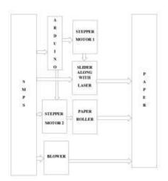
It mainly follows a paper rolling and a slider mechanism. Two aluminium channels are also provided along with a foam board basement for the smooth paper movement. A paper roller is mounted to intiates the forward paper movement. The roller mechanism comprises of a stepper motor paper roller, timing belt and gears. The laser unit is mounted on a sliding mechanism which is designed
