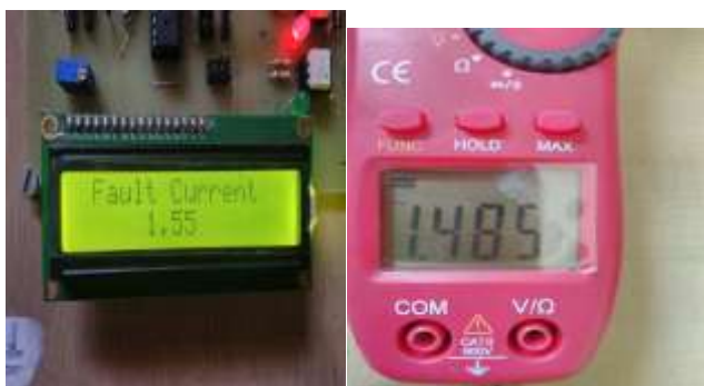
Fig -4.1: Current Value at fault condition
