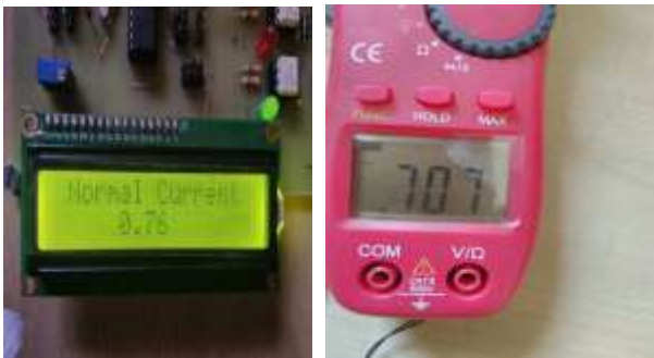
Fig -4: Current Value at Normal Condition
