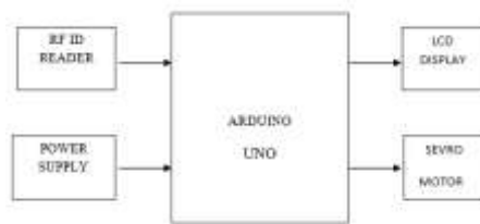
Fig-5: Receiver unite for speed breaker
