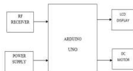
Fig-3: Receiver module Block diagram
