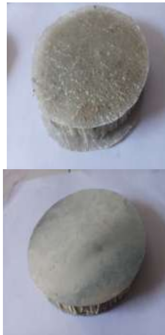
Fig-5: Face sheets of Aluminum and Glass fiber.
