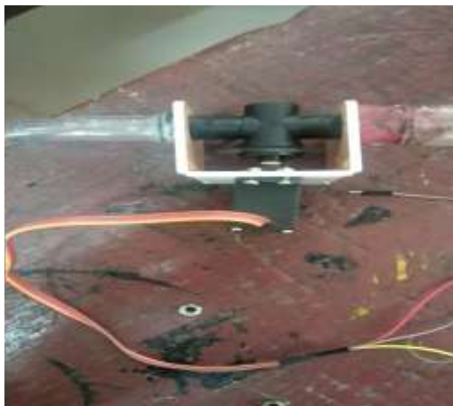
Fig- 18: Servo motor controlled outlet valve
