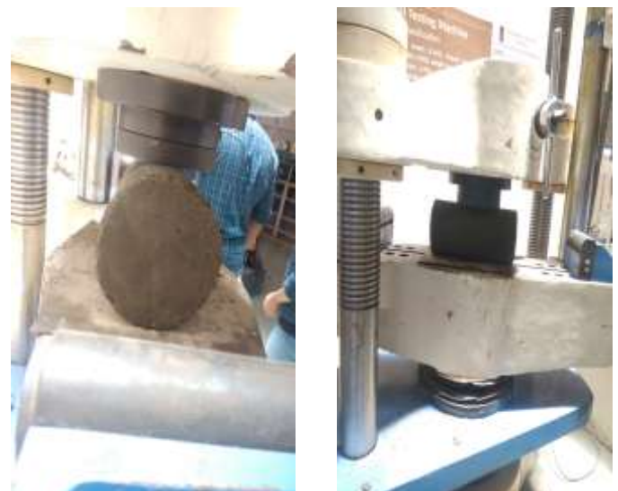
Fig 3. Split Tensile Strength of SSA concrete cylinder.
