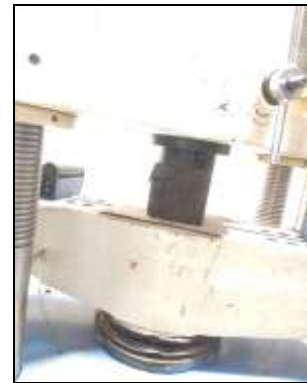
Fig 2. Compression Testing of SSA concrete cube.
