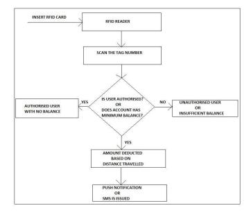
Fig 2: Flow diagram of the system
