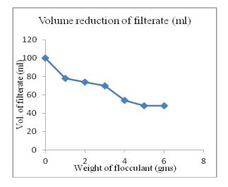
Fig.-7: Vol. of filtrate vs. weight of flocculant
