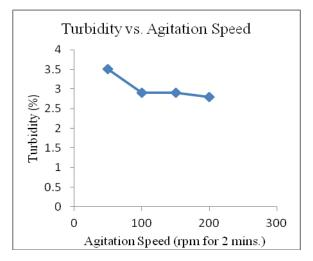
Fig.-23: Turbidity vs. Agitation Speed
