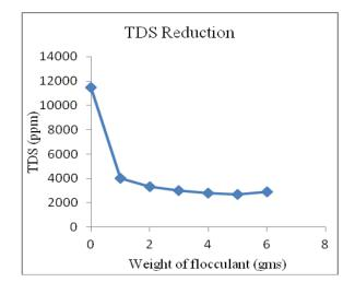
Fig.-3: TDS vs. weight of flocculant
