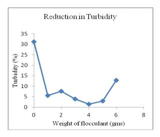
Fig.-6: Turbidity vs. weight of flocculant
