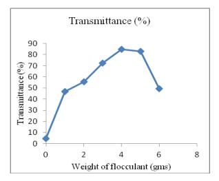
Fig.-4: Transmittance vs. weight of flocculant
