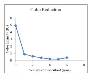
Fig.-5: Color intensity vs. weight of flocculant
