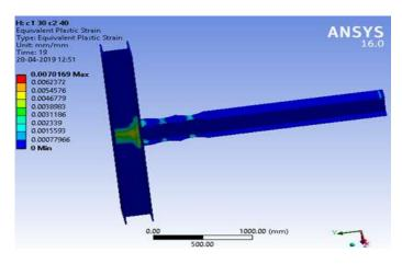
Fig -3: Equivalent strain distribution in DRBS-C<sub>1</sub>30
