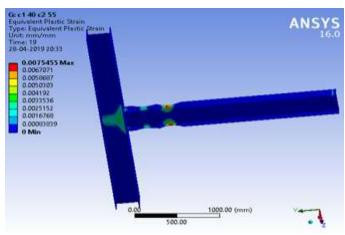
Fig -5: Equivalent strain distribution in DRBS-C<sub>2</sub>55
