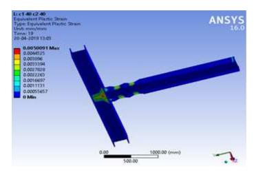
Fig -4: Equivalent strain distribution in DRBS-C<sub>1</sub>40
