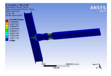
Fig -6: Equivalent strain distribution in DRBS-C<sub>2</sub>60
