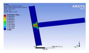
Fig -2: Equivalent strain distribution in OBC
