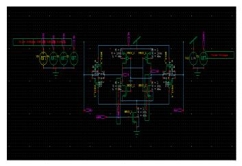
Fig -7: Schematic Diagram of Transmission Gate VMSA
