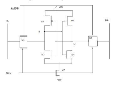
Fig -4: Transmission Gate VMSA [3]
