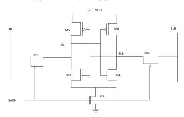
Fig -1: Cross-coupled voltage mode SA [4]
