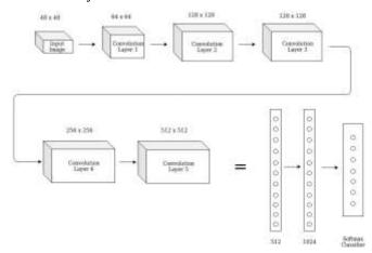
Fig. (1): 5-Layered CNN Architecture
