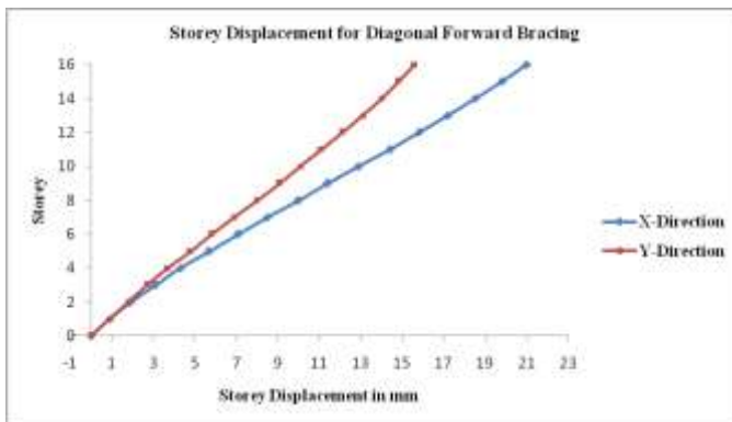
Figure 8: Storey displacement for Diagonal forward bracing along Y direction
