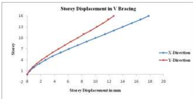
Figure 7: Storey displacement for V bracing along Y direction
