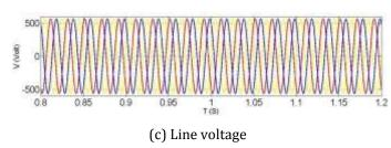
Fig 7 - Results funder L-L-L-G fault with DVR protection
