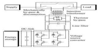
Fig 2 - Schematic arrangement of DVR
