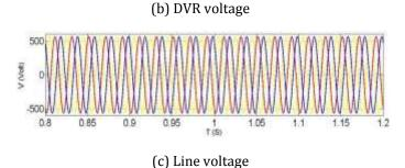
Fig 6 - Results under L-L-G fault with DVR protection
