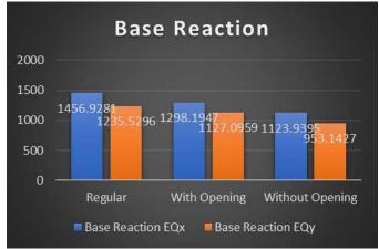
**Graph -1**: Graph for base shear for regular structure, with shear wall and shear wall with opening.
