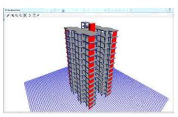
Fig -4: Building with Shear wall Having Opening.
