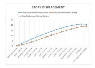
**Graph -3**: Graph for story displacement for regular structure, with shear wall and shear wall with opening.
