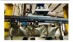
Fig -6: Arrangement of Dial Gauges and Beam loaded into the setup
