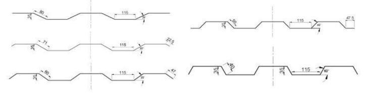
Fig -4: Detailed Diagrams of Web Profiles with angle of corrugation as 25°, 30°, 35°, 45° and 60°
