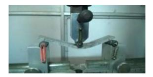
**Figure 4.** Flexural testing of the specimen.
